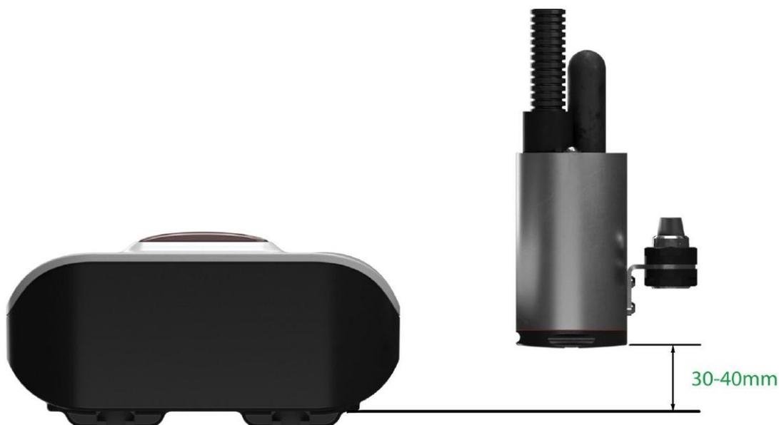
The difference in height between the lowest jet orifice and the base of the machine **must** be between 30mm and 50mm. Over 50mm will starve the head, less than 30mm will cause the machine to weep.
