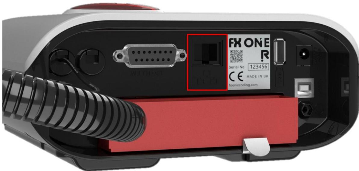
An extension to wired Ethernet is wireless (WiFi). Foenix Coding do not directly support WiFi however the customer can use a Wireless Bridge to provide the link between the network and physical RJ45 socket for the printer.
